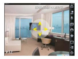
Support PTZ dome control (includes preset function) and regular zoom in/out, iris adjusting and etc.; easy gestures control to realize EPTZ function (for non-dome cameras).
